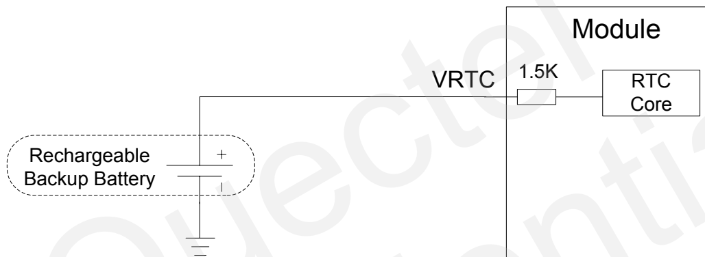
Figure 15: RTC Supply from a Rechargeable Battery
