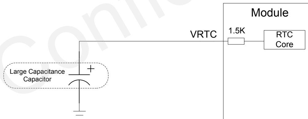
Figure 16: RTC Supply from a Capacitor
