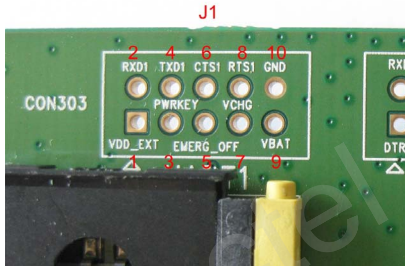
Figure 13: J1 test points
