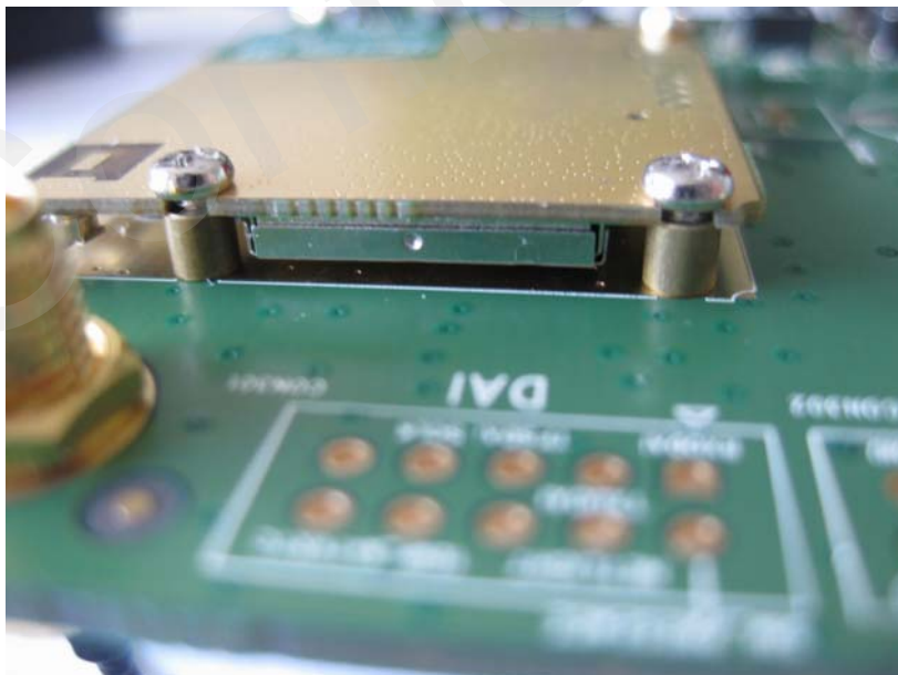
Figure 18: Bolts to support EVB
