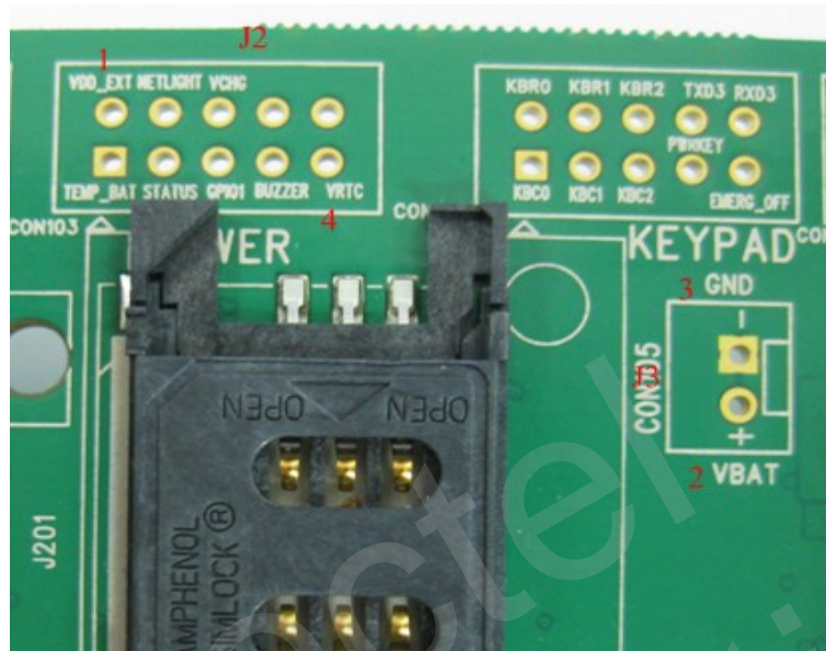
Figure 12: Power test points
