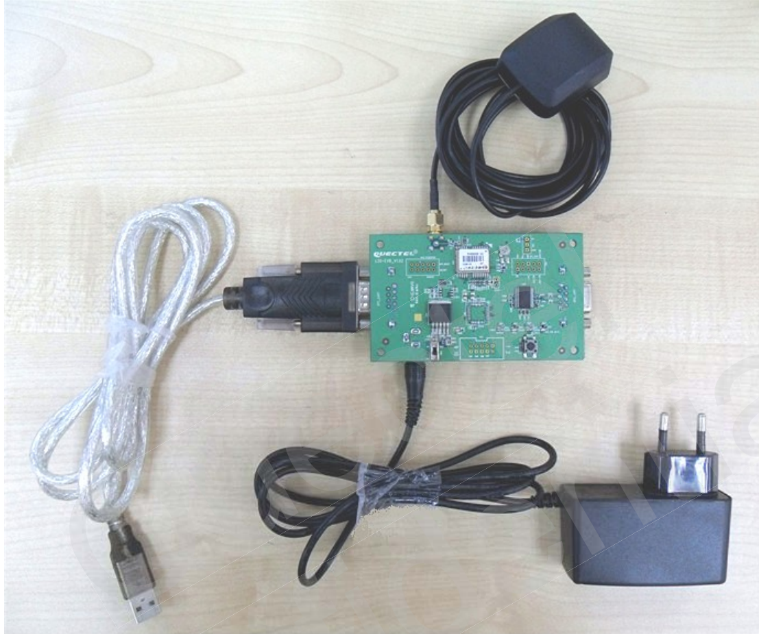
Figure 10: EVB and accessory equipments
