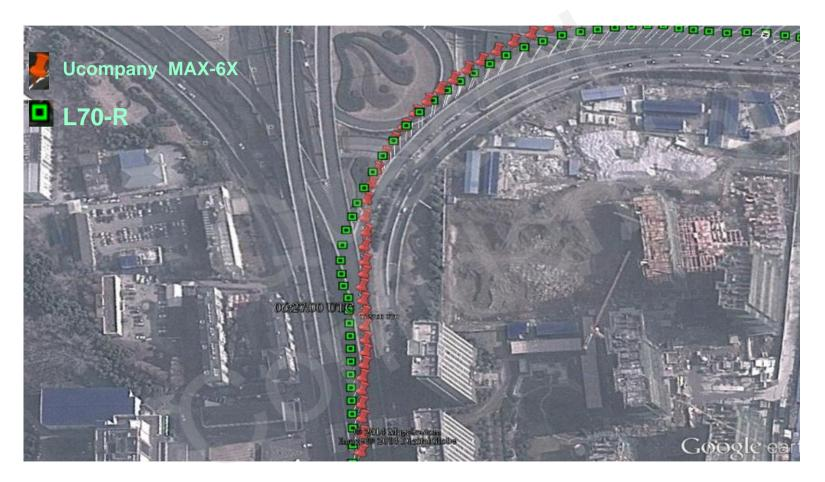
When driving across overpass and making a turn, L70-R module can still capture the accurate tracking data. But Ucompany module has a small drift.
