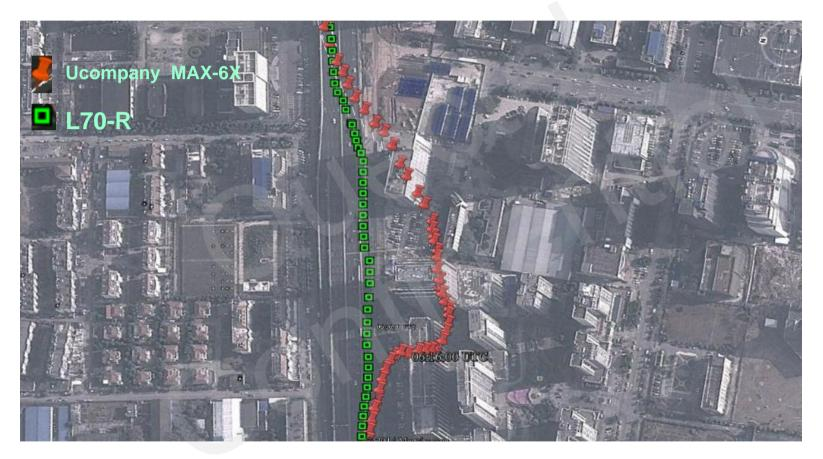
When driving under the overpass, L70-R module shows its excellent performance. But Ucompany's module has a bigger drift.
