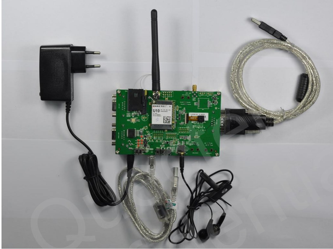
Figure 54: EVB and accessories equipment
