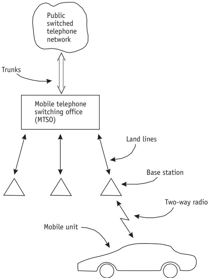
**Figure 9.5** The mobile unit communicates by two-way radio with the base station. The base stations all communicate over landlines with the mobile telephone switching office (MTSO), which then maintains communication with the public switched telephone network (PSTN).
