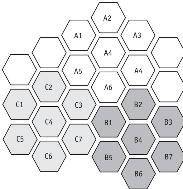
**Figure 9.1** Cells are organized into clusters, with most cellular systems using seven cells per cluster. The clusters are then repeated over and over again to cover the whole geographic area served by the system. Although the cells are depicted as hexagons, their actual shape is quite irregular and depends on the terrain and radio propagation.
