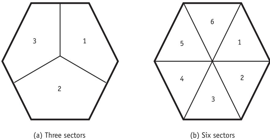
**Figure 9.3** With sectorization, a directional antenna is beamed to divide a cell coverage into sectors, like wedges in a pie. Three (a) and six (b) sectors are typical. The narrow beam of the radio signal minimizes multipaths and can be more powerfully concentrated, thereby extending its range.
