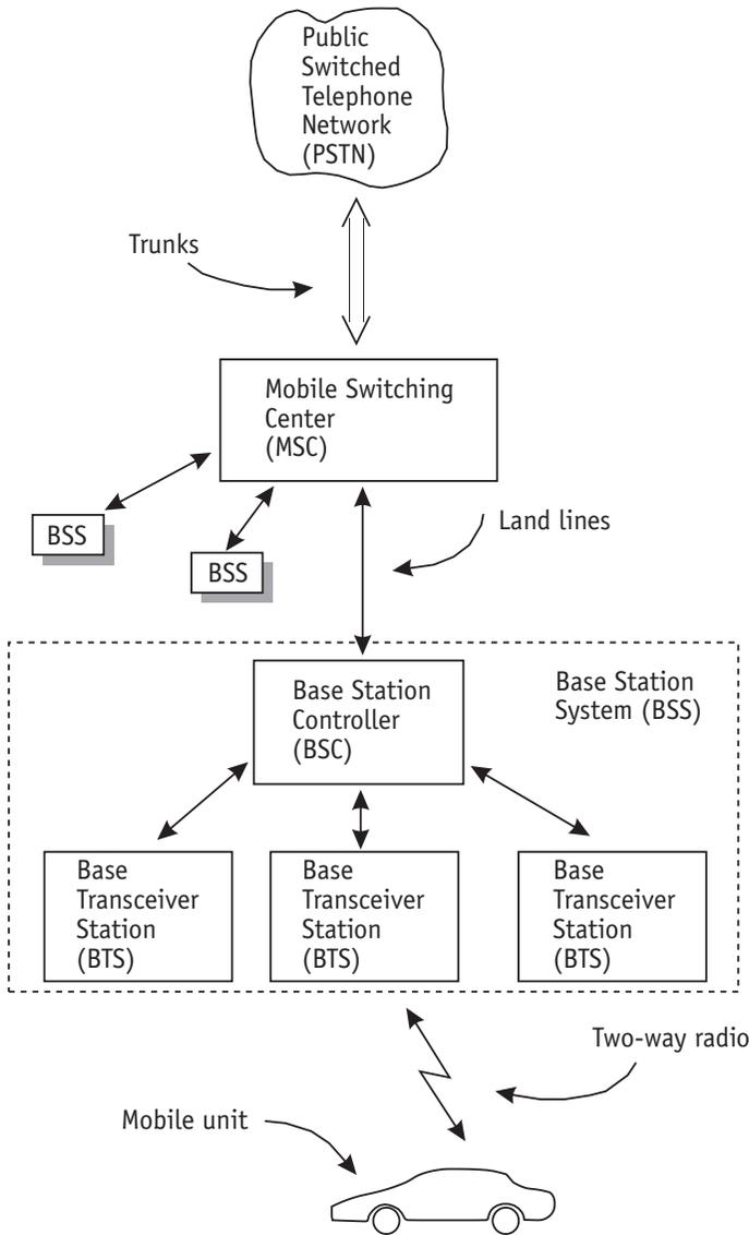
**Figure 9.7** A mobile unit communicates by two-way radio with a base antenna at the base transceiver station (BTS). A number of BTSs are monitored and controlled by a BSC. The BSC and its BTSs form a base station subsystem (BSS). A number of BSSs are controlled and monitored by the mobile switching center (MSC), which also is the gateway to the public switched telephone network (PSTN). The MSC has access to various databases that contain information about the mobile users.
