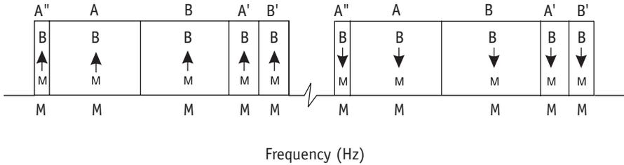
**Figure 9.6** Two radio-frequency bands are used for cellular telephone service in the 900-MHz bands by the AMPS system. The band from 824 MHz to 849 MHz is used for transmission from the mobile unit to the base station (the uplink) and is shared by the A and B systems. The band from 869 MHz to 894 MHz is used for transmission from the base station to the mobile unit (the downlink) and is likewise shared by the A and B systems.
