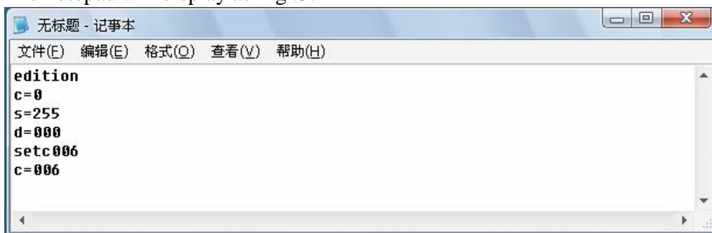
Fig.3 Input the command setc006 slowly and change the channel to 6
