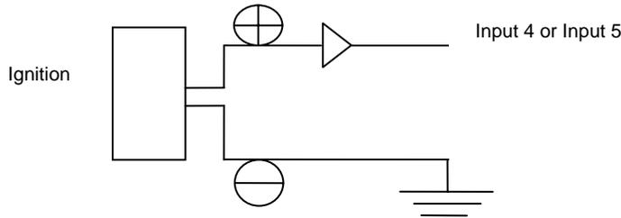
3. Detecting Lock Status of Car's Door or Trunk(Car Boot): Locked or Unlocked - Input 4 / Input 5
