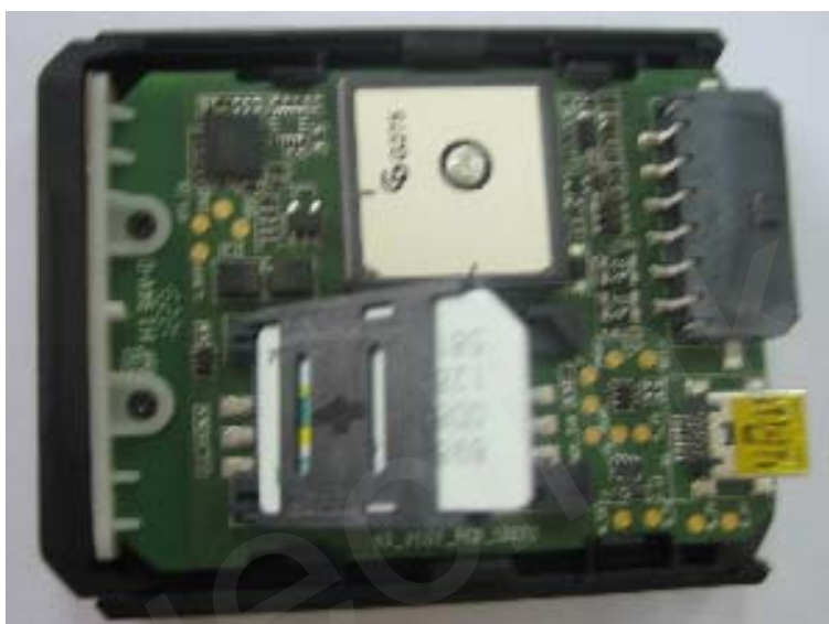
Figure 5. SIM Card Installation
