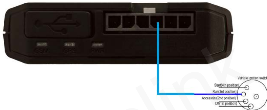
Figure 7. Typical Ignition Detection
