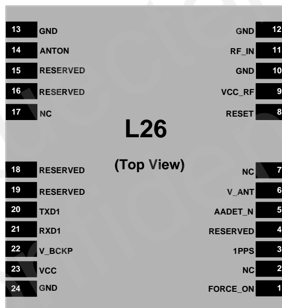
Figure 2: Pin Assignment
