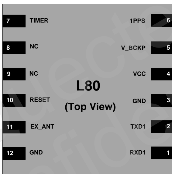
Figure 2: Pin Assignment
