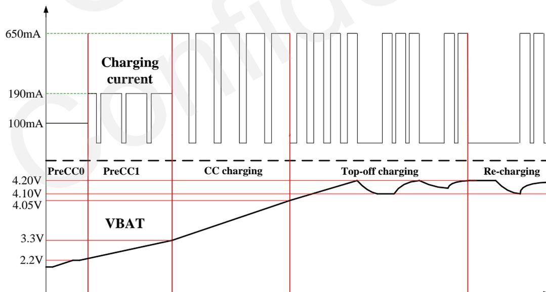
Figure 4: Normal charging process diagram
